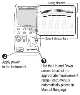
Tuning is shown on the display using tuning needles and zone indicator bars. The tuning needles (at the top of the display) are now zoomed in to enhance laser tuning. For detailed information about Tuning mode, refer to the *FieldMaxII-TO User Manual*.
