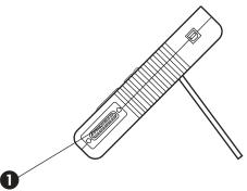
Connect a thermopile or optical sensor to the FieldMaxII-TO 25-pin connector.
