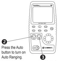
Block the beam and then press the Zero button to set the baseline for your new measurement.
