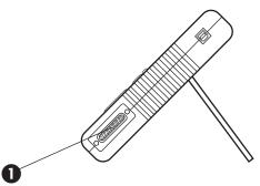
Connect a thermopile or optical sensor to the FieldMaxII-TO 25-pin connector.
